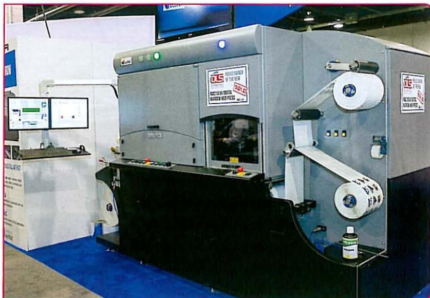
*The NW210 UV inkjet press from INX incorporates a Spartanic laser die-cutting station*
