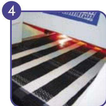
After printing the sheets pass under an infra red heating unit which causes the droplets to flow together and smooth the surface. The actual gloss level is determined by the number of droplets per pixel applied by the printhead.
