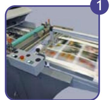
The offset style pile feeder and the sidelay guide can be set up to position the sheets precisely under the print head. The MGI front end software then allows exact positioning of the image over the sheet.
