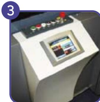
The control panel lets you adjust the sidelay guides, for position and skew, and the set up the feeder, conveyor, IR and UV processes, as well as starting and stopping production.
